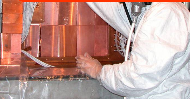
closing the Cu box housing the detectors
