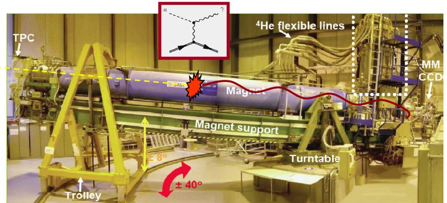
CAST is using a decommissioned prototype superconducting LHC dipole magnet to detect solar axions:
