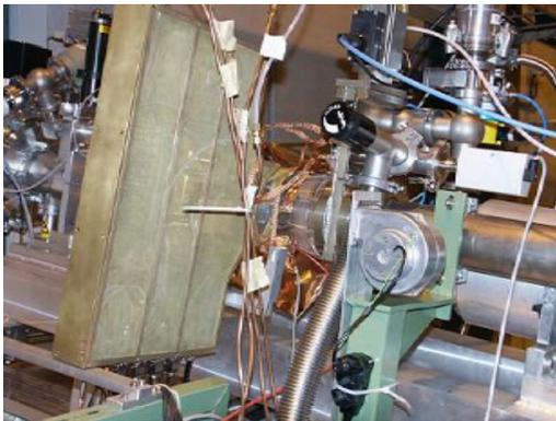
The X-Ray Telescope is focusing a  $\varnothing 43$  mm x-ray beam to  $\varnothing 3$ mm
