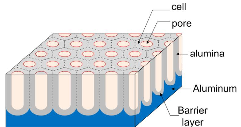
A schematic representation of a close-packed array of columnar alumina units. The barrier layer as well as the Aluminum substrate can be removed in a post procedure following the anodization.
